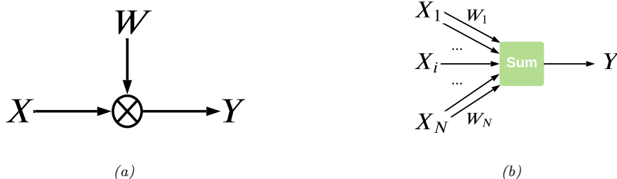
Figure 16.1: An artificial “neuron”, the most basic building block of a DNN. (a) The output y is a weighted combination of the inputs \mathbf{x} , where the weights vector is denoted by \mathbf{w} . (b) Alternative depiction of the neuron’s behavior. The bias term b can be emulated by defining w_N = b and X_N = 1 .
