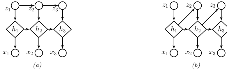
Figure 29.43: Recurrent state-space models. (a) Prior is first-order Markov, p(\mathbf{z}_t|\mathbf{z}_{t-1}) , but observation model is not Markovian, p(\mathbf{x}_t|\mathbf{h}_t) = p(\mathbf{x}_t|\mathbf{z}_{1:t}) , where \mathbf{h}_t summarizes \mathbf{z}_{1:t} . (b) Prior model is no longer first-order Markov either, p(\mathbf{z}_t|\mathbf{h}_{t-1}) = p(\mathbf{z}_t|\mathbf{z}_{1:t-1}) . Diamonds are deterministic nodes, circles are stochastic.
