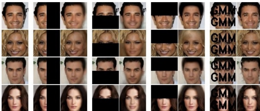
Figure 28.14: Illustration of image imputation using an MFA. Left column shows 4 original images. Subsequent pairs of columns show an occluded input, and a predicted output. Generated by mix_ppca_celebA.ipynb . Adapted from Figure 7b of [RW18]. Used with kind permission of Yair Weiss.
