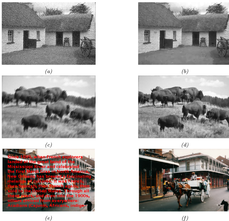
Figure 28.4: Example of recovering a clean image (right) from a corrupted version (left) using MAP estimation with a GMM patch prior and Gaussian likelihood. First row: image denoising. Second row: image deblurring. Third row: image inpainting. From [RW15] and [ZW11]. Used with kind permission of Dan Rosenbaum and Daniel Zoran.
