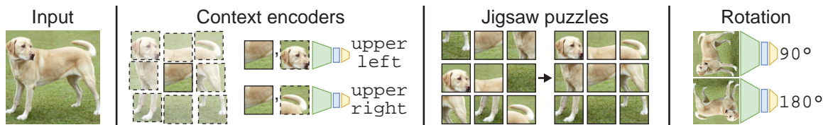
Figure 32.4: Transformation prediction involves training neural networks to predict a transformation applied to the input. Context encoders predict the position of a second crop relative to the first. The jigsaw puzzle task involves predicting the way in which patches have been permuted. Rotation prediction involves predicting the rotation that was applied to the input.
