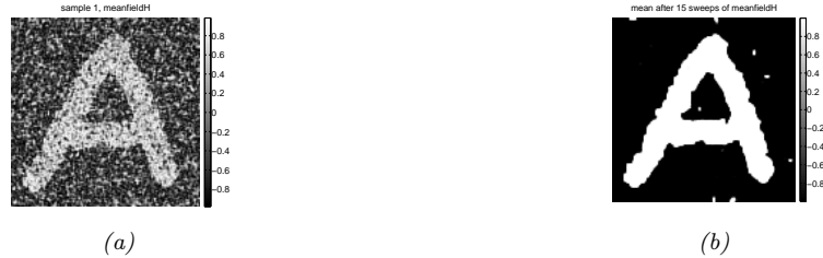
Figure 4.27: Example of image denoising using mean field variational inference. We use an Ising prior with W_{ij} = 1 and a Gaussian noise model with \sigma = 2 . (a) Noisy image. (b) Result of inference. Generated by ising_image_denoise_demo.ipynb .
