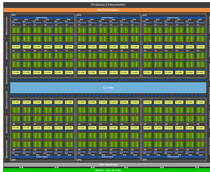
Fig. 13.4.8 NVIDIA Turing architecture (image courtesy of NVIDIA)
